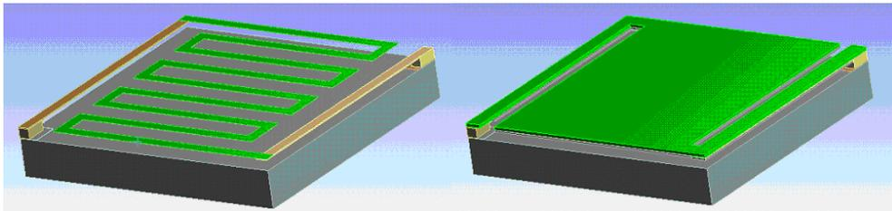
Fig. 1 Microbolometer structure without isolating membrane (left) and with isolating membrane (right)
