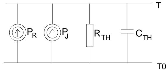
Fig. 2 Equivalent electrical model
