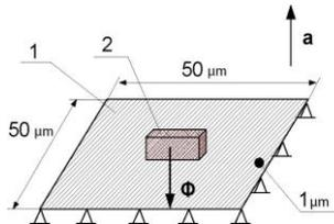
Fig. 1 Microaccelerometer's calculation scheme.
