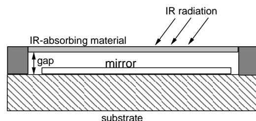
Figure 1: Simplified cross-section of a microbolometer.
