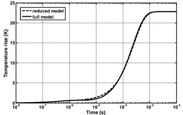
Figure 4: Simulated heating by sensor current.
