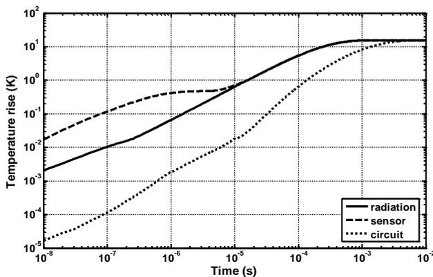
Figure 2: Normalized heating curves simulated with full distributed model.
